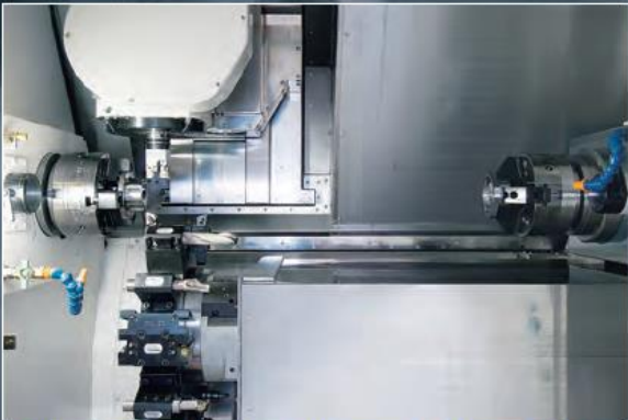
Simultaneous turning with upper and lower tools. Thanks to tool spindle orientation, a multi-tool holder can be used.
