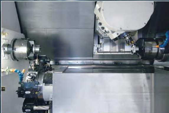
Milling / Tool spindle milling on right side spindle, lower turret machining on the L side. Through compact turret and tool spindle, tooling interference is minimized.
